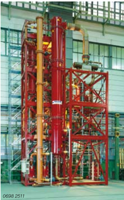
The pressure swing distillation system for hydrochloric acid produces pure HCl gas without any contamination through by-products
