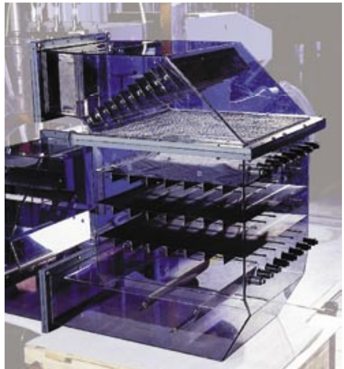
Model mixer set up with Sulzer SMV Mixer
